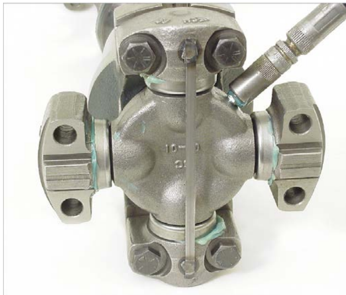
Fig. 4 Seals allow grease to bleed so lubricant can flow through all trunnions
