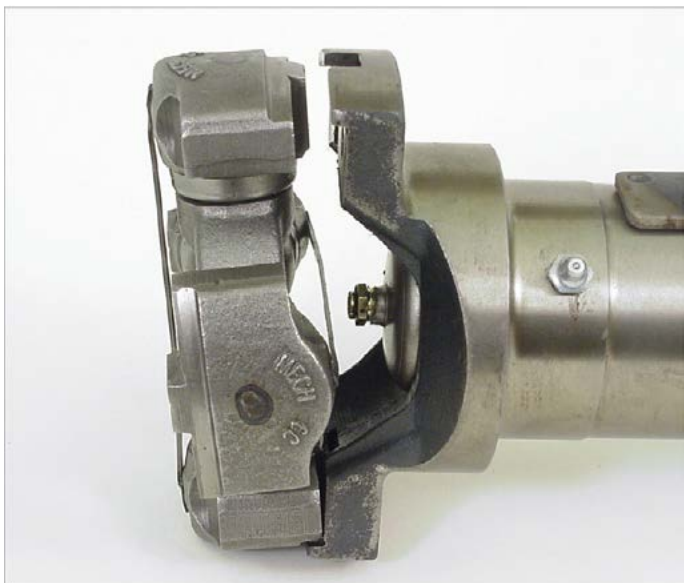
Fig. 1 Insertion of key and pilot of bearing into yoke
