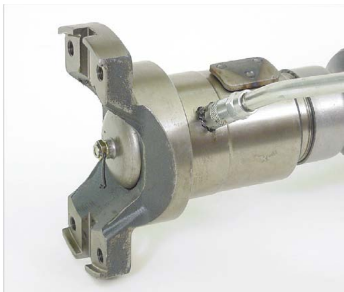
Fig. 3 Grease appears from vent hole
