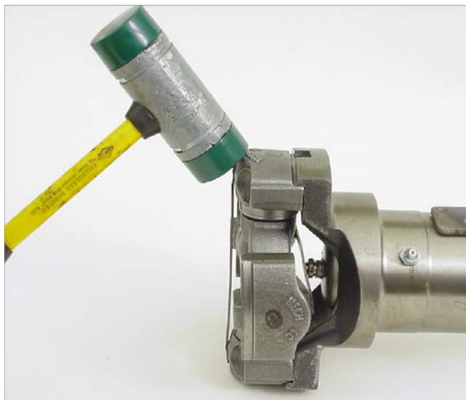
Fig. 2 Opposite bearing installed
